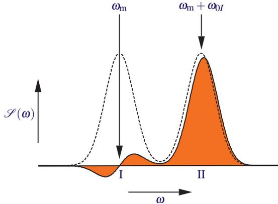
Figure 3: ESR spectrum consisting of two separated ESR lines I and II. Spectral diffusion is fast compared to electron spin-lattice relaxation, and Provotorov's theory describes the saturation of the ESR signal. Triple spin flips tend to equalize the inverse electron non-Zeeman temperature and the inverse nuclear spin temperature.
