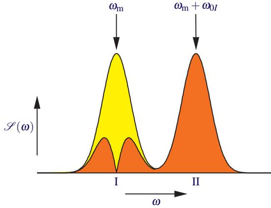
Figure 2: ESR signal displaying two separated ESR lines I and II. A hole is burnt at the microwave frequency  $\omega_m$ . Triple spin flips at the frequencies  $\omega_m$  and  $\omega_m \pm \omega_{0I}$  contribute to enhancement of the nuclear spin polarization. All other triple spin flips contribute to nuclear spin-lattice relaxation.
