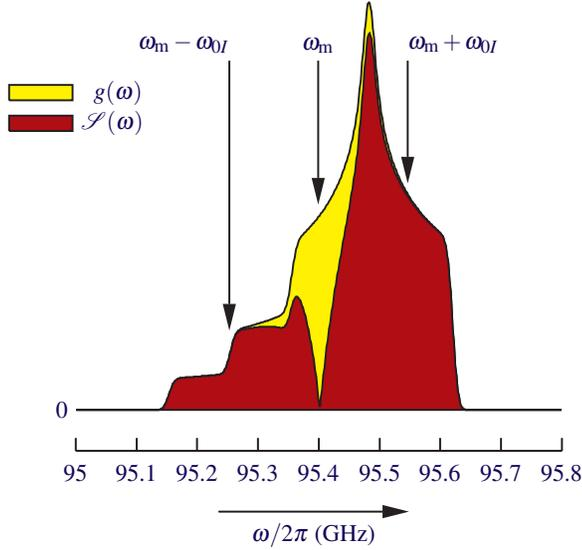
Figure 1: Simulation of the ESR signal resulting from the simultaneous action of the microwave field, spectral diffusion and electron spin-lattice relaxation, as shown in Figure 5.10 of *EofDNP*. For the details, see the caption of that figure. Triple spin flips involving electron spins with a resonance frequency near  $\omega_m$  and  $\omega_m \pm \omega_{0I}$  contribute to enhancement of the nuclear spin polarization. All other triple spin flips contribute to nuclear spin-lattice relaxation.
