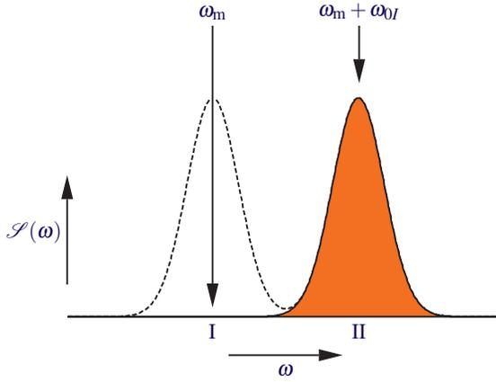
Figure 5: ESR spectrum consisting of two separated ESR lines I and II. Spectral diffusion is fast within each individual ESR line, but slow across the full ESR spectrum. When the separation of the two ESR lines is near the NMR frequency  $\omega_{0I}$ , the cross effect governs the enhancement of the nuclear spin polarization in DNP and nuclear spin-lattice relaxation.
